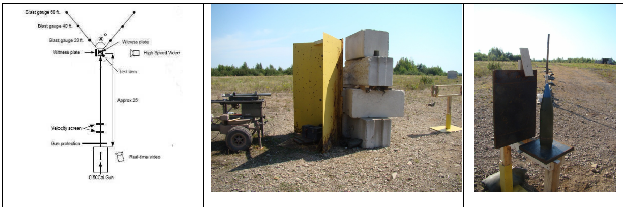
Figure 2 – Bullet impact set-up and views of some equipment
