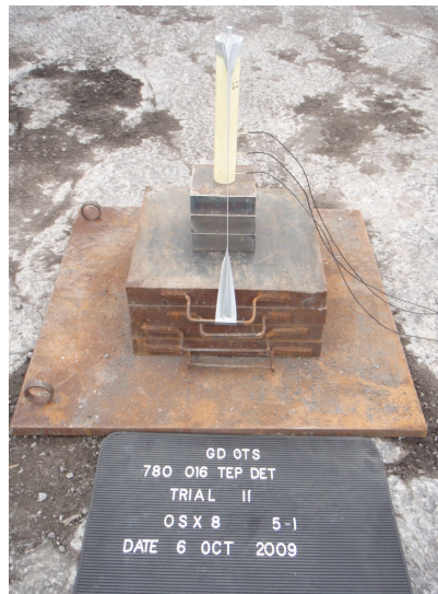
Figure 1: Detonation velocity and plate dent test set-up
