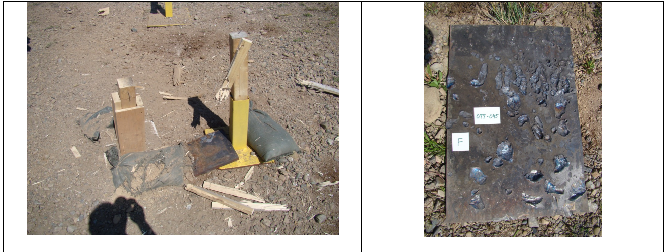
Figure 4 – Test set-up and side witness plate after composition B bullet impact test
