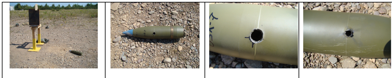
Figure 5 – Test set-up and recovered projectile from IMX-104 (OSX-7) bullet impact test
