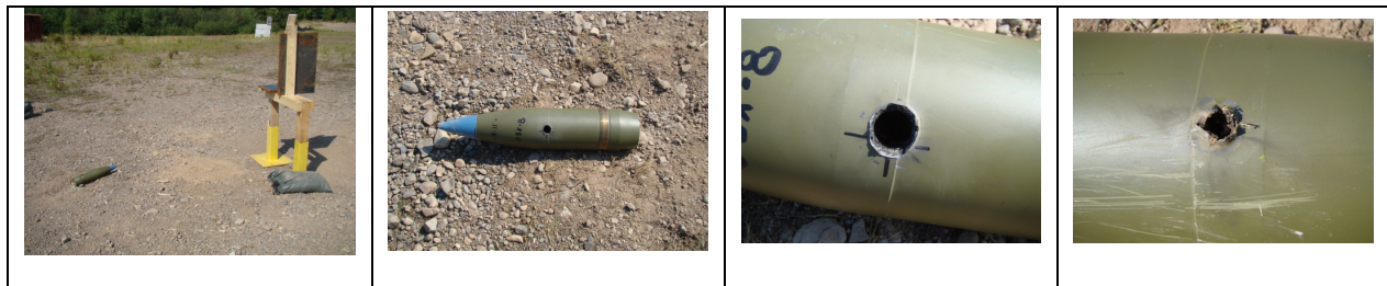
Figure 6 – Test set-up and recovered projectile from PAX-48 (OSX-8) bullet impact test
